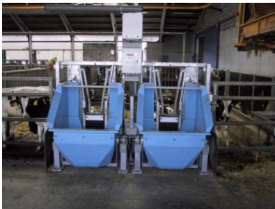
Insentec automated feeders used to record individual feed intake
