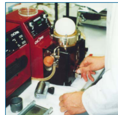
Chopin Alveograph showing stage 5 - air being pumped into dough
