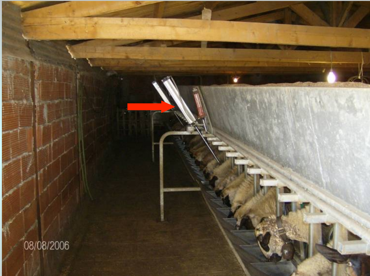
Figure 11. The hydraulic lifting system of entrapment in milking machines of the fast exit type with automatic feeders 23
