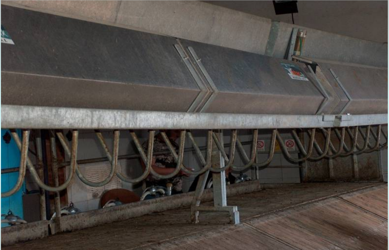
Figure 13. The entrapment system is lowering after the exit of the group of animals
