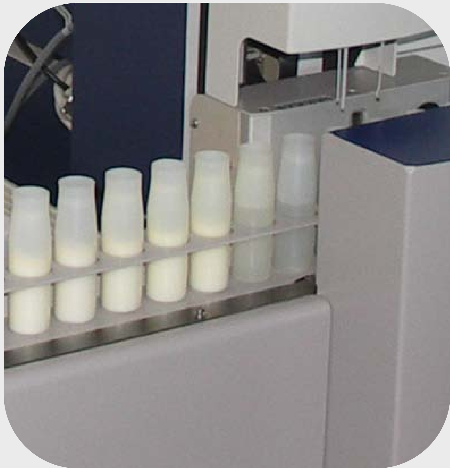
Fig.2: SCC of the unpreserved samples was measured with the Fossomatic 5000 (FOSS)
