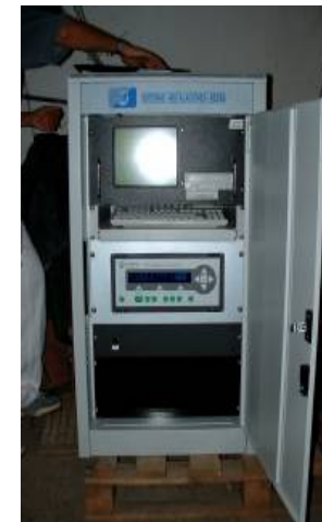
Measurement system: Innova 1312 (Sir S.A., Madrid)
