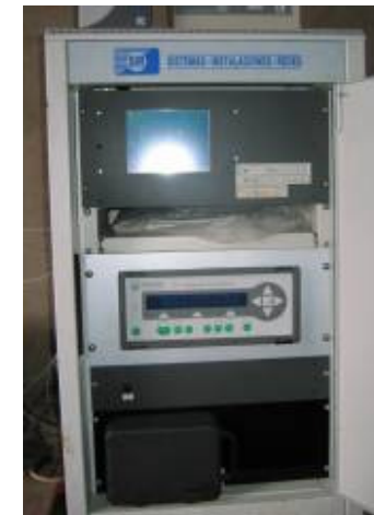
Measurement system: Innova 1312 (Sir S.A., Madrid)
