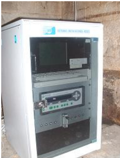
Measurement system: Innova 1312 (Sir S.A., Madrid)
