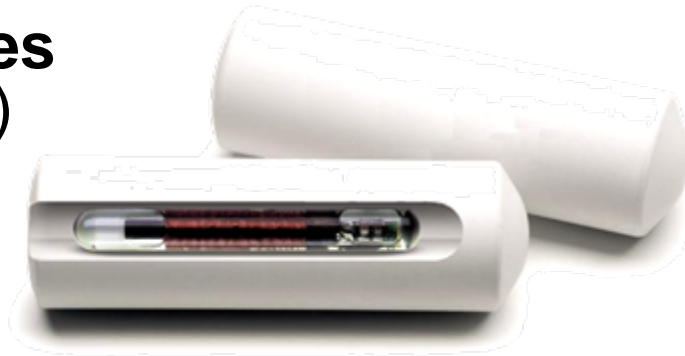
Glass encapsulated transponder (32 × 3.8 mm)
