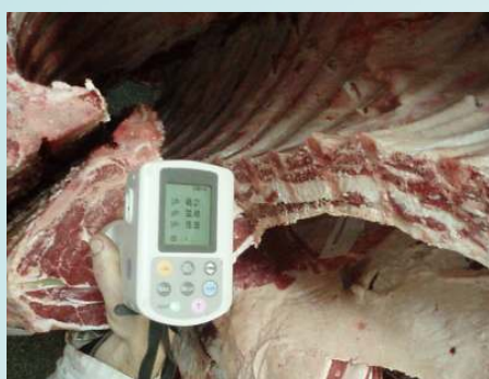
Fig. 1: Colour measuring (Minolta Chroma Meter CR-410)
