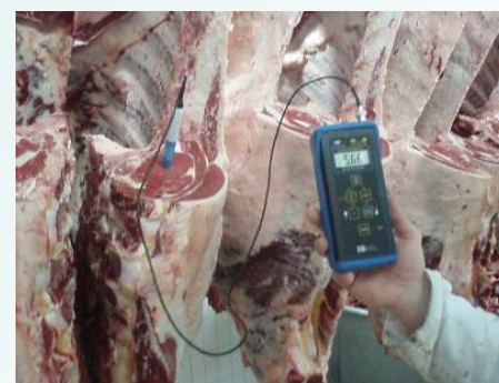
Fig. 3: pH value measurement (pH meter IQ 150)
