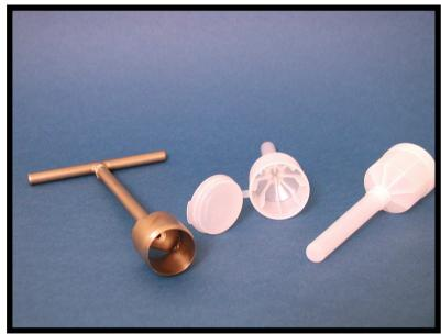
A special cylinder knife and special containers secure the same treatment of all samples
