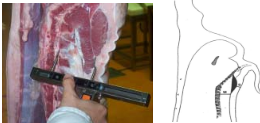
Fig. 1: Example of electronic caliper and the measuring locations
